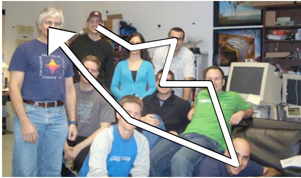
Figure 4: "Find Faces" option in Image Viewer creates a Hamiltonian path through each face of a photograph. Scrolling with CAS widget follows this path (as shown by the arrow).
